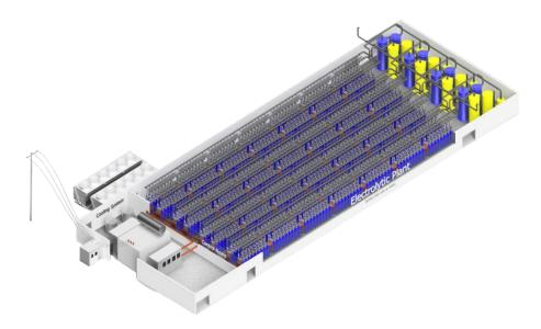
Hydrogen Optimized's patented **RuggedCell™** unipolar alkaline water electrolyzers are designed for the lowest levelized cost of clean hydrogen at large scale. Building on the proven Stuart technology platform, the system's attributes include **dynamic power response**, **20 year lifespan** with minimal efficiency loss, **low-cost on-site maintenance**, and **no Iridium and PFAS "forever chemicals"**.
